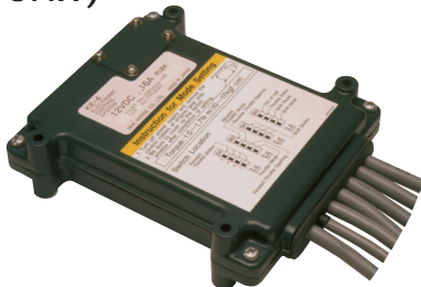
ECU (ELECTRONIC CONTROL UNIT)
