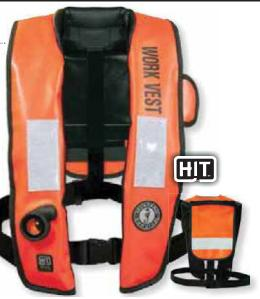
Hydrostatic Inflator Technology (HIT™) · ises a pressure valve that will inflate the PFD if immersed in 4"or more of water pressure. No more inadvertent inflation due to high humidity, rain, or splash.
