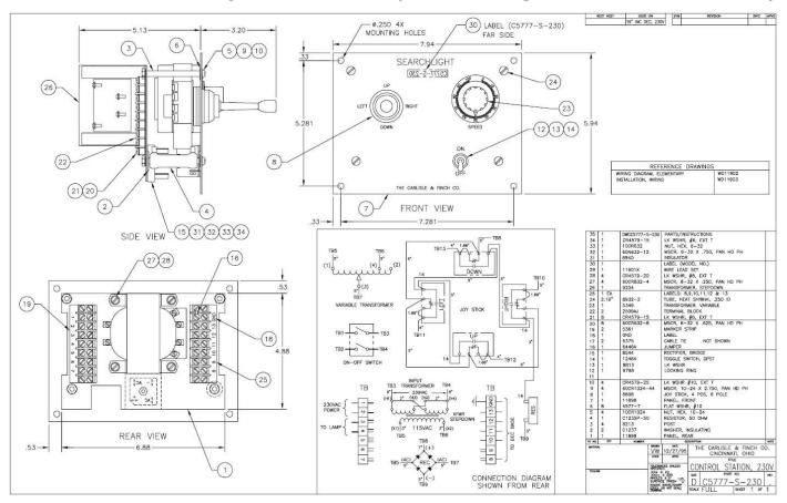
Model 8779X-S Joystick Controller (Used for Multiple Points of Control, 115V)
