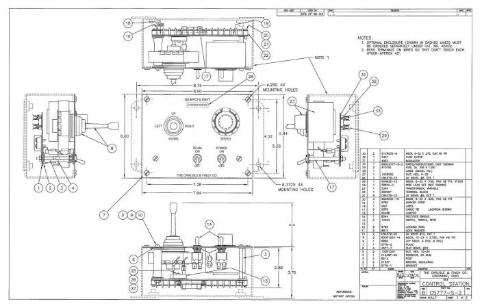
Model C5777-S-230 Joystick Controller (Used for Single Point of Control, 230V)
